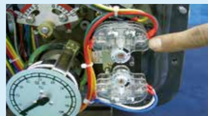
Limit switch inspection
